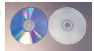
Comparison of data bearing disc and disc run through DX-CD2
