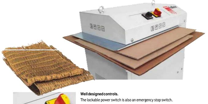
**Model PacMaster S**: There is a rotary switch to turn the machine on and off and into reverse.
