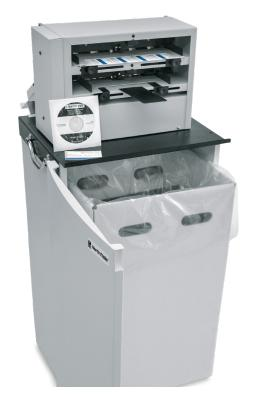
Handles sheet sizes from 65# to 100# cover, 177 to 270 gsm Creates up to 360 cards per minute
