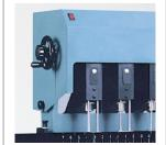
The drilling heads are easily adjustable with the calibrated hand cranks.
