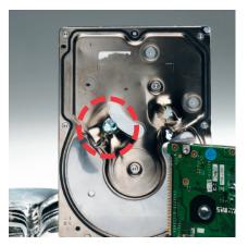
Punching a hole completely through the drive damages all components (metal housing, disk, and electronic parts) irreparably, rendering it unreadable.
