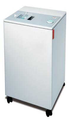
Comprehensive SPS safety package: Easy Switch control element uses illuminated color codes and symbols to indicate operational status and functions as an emergency stop switch; electronically controlled, transparent safety shield in the feed opening; automatic stop after punching; automatic power cut-off when cabinet is opened or collection bin is full; double protection against overheating.
