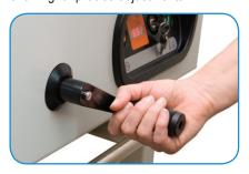
Hand Crank Back Gauge Adjustment
