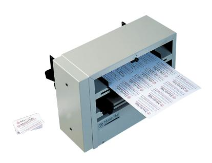
12-up machine that cuts 8.5" x 11" sheets into three strips of 3.5" x 8.5" on the first pass
