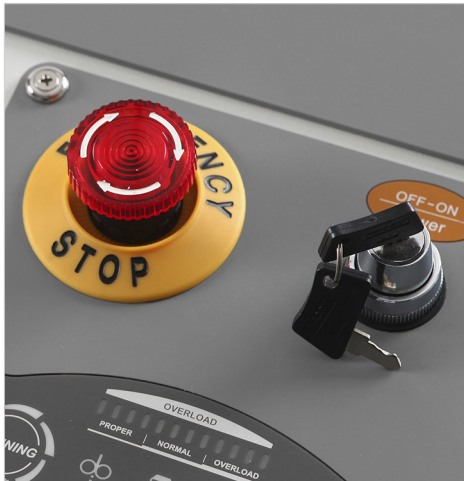
Safety features include emergency stop button and key lock to prevent unauthorized use.
