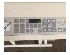
MEMORY KEYS The touch panel sets up 6 standard folds automatically at the touch of a button. Up to 30 custom folds can be stored in memory.
