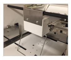
**BELT FEED SYSTEM** A belt fed, air suction system allows trouble-free feeding of coated stock.
